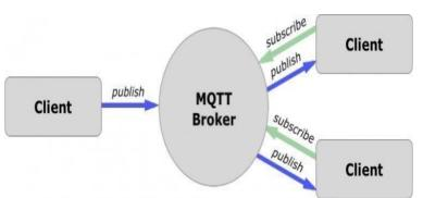
Fig. 1. Operation.in MQTT protocol
