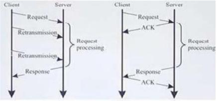
Fig 3. Message exchange phase in AMQP
